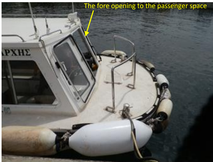
Figure 5: DRAGON TAXIARCHIS bow arrangement and the fore opening leading to the closed passenger accommodation area.
