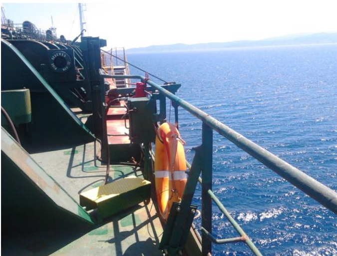
Figure 6: The lifering located close to the accommodation ladder control post.
