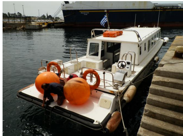
Figure 9: The aft control station
