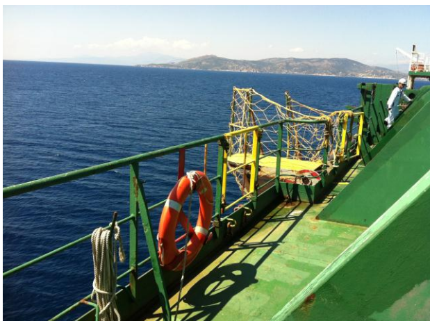
Figure 7: The lifering with rope which was placed close to the Stbrd accommodation ladder towards the fore.
