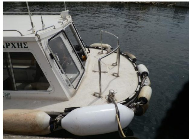
Figure 11: The fore embarkation deck with the weather tight opening for the access to the passenger area and the railings.
