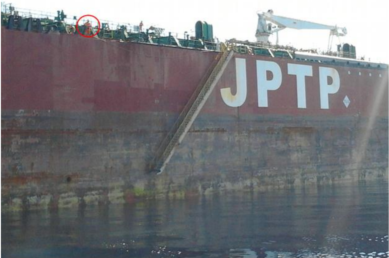
Figure 4: The Starboard accommodation ladder at ROYAL OAK main deck and the position of the ladder's control post where Bosun was standing.
